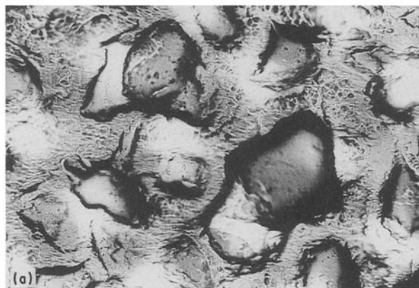
Figure 5 Optical phase contrast photomicrograph of PVC surface grafted using 5% monomer concentration at different NVP: HEMA combinations at 0.25 Mrad: (a) N25: H75, (b) N50: H50 and (c) N75: H25.
